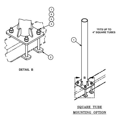
**TOLERANCE NOTES** TOLERANCES ON DIMENSIONS, UNLESS OTHERWISE NOTED ARE: SAWED, SHEARED AND GAS CUT EDGES (\$ 0.030") DRILLED AND GAS CUT HOLES (\$ 0.030") - NO CONING OF HOLES LASER CUT EDGES AND HOLES (\$ 0.010") - NO CONING OF HOLES BENDS AND ANGLES ARE ± 1/2 DEGREE ALL OTHER MACHINING (± 0.030") ALL OTHER ASSEMBLY (± 0.060")
